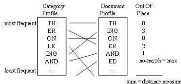
Fig. 5. An illustrative example for the calculation of n-gram profile distance between documents.
